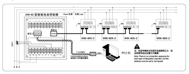
WSK-8DF-Z 系列与 JKW-8DF 型控制器组成混合补偿系统典型应用接线图 Typical application wiring diagram of hybrid compensation system composed of WSK-8DF-Z series and JKW-8DF controller
